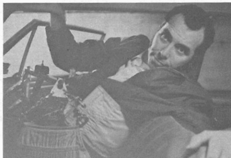
#9 Wolfe lift to transfer from wheelchair to car. Overhead bar (not shown) helps to slide across to driver's seat.
