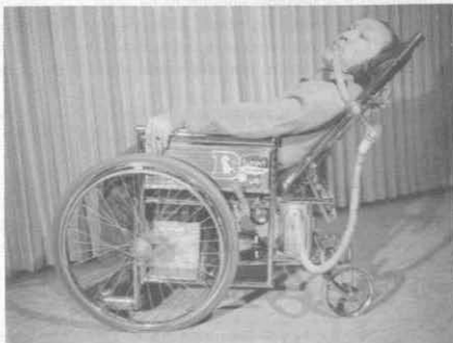
During daytime hours W. Sunny Weingarten uses a LPS positive pressure respirator with a mouth tube. The unit will run over 24 hours on one charged auto battery and has a built-in charger.
