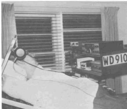
Cantilever rack holds CB and amateur radio equipment over rocking bed.
