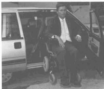
Figure 2. Carchair system with chairlift in operation
