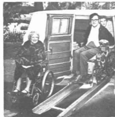
Fig. 6 Homemade wooden ramp.
