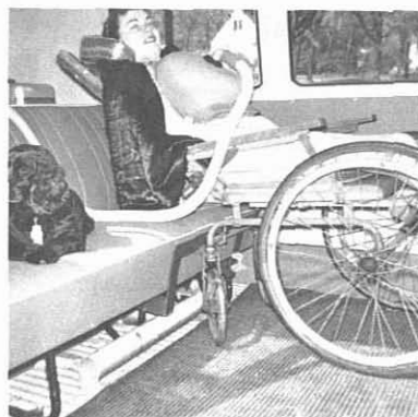
My chair is anchored by steel pins to the framework which is attached to the back seat.
