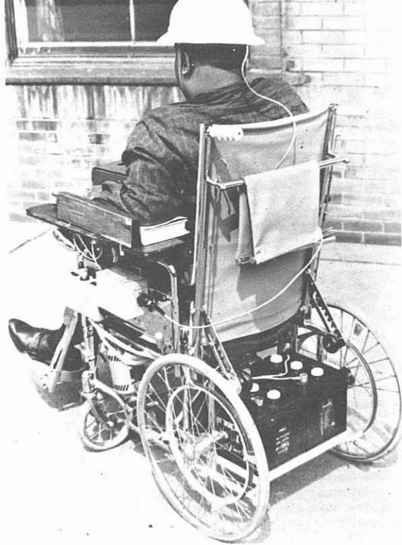
The logic box mounted on the chair and the wire leading to it from the hat can be seen in this photograph. The batteries are standard equipment supplied with the wheelchair and power all the equipment for one day, from an over-night charge. Automatic safety features prevent unintended operation of the control system, as when using the mouthstick or sneezing.
