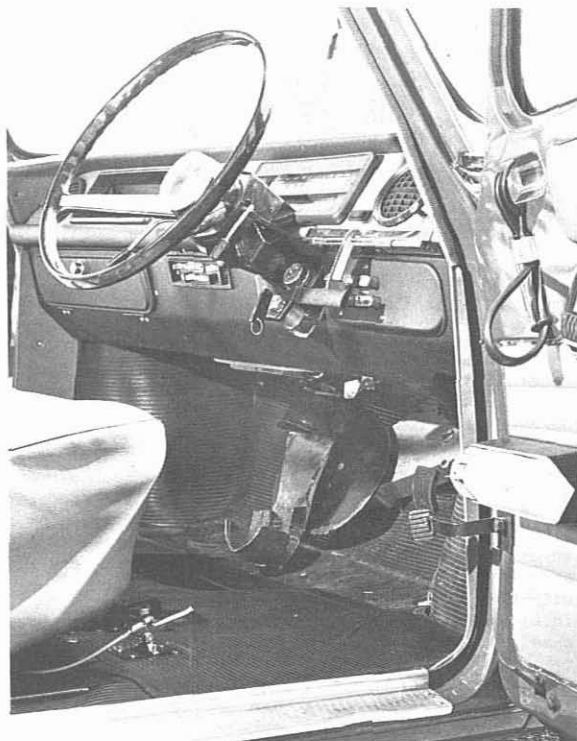
This photograph shows the steel shoe by which the car is steered. It will be seen that other controls have been converted to use by the right foot or knee.
