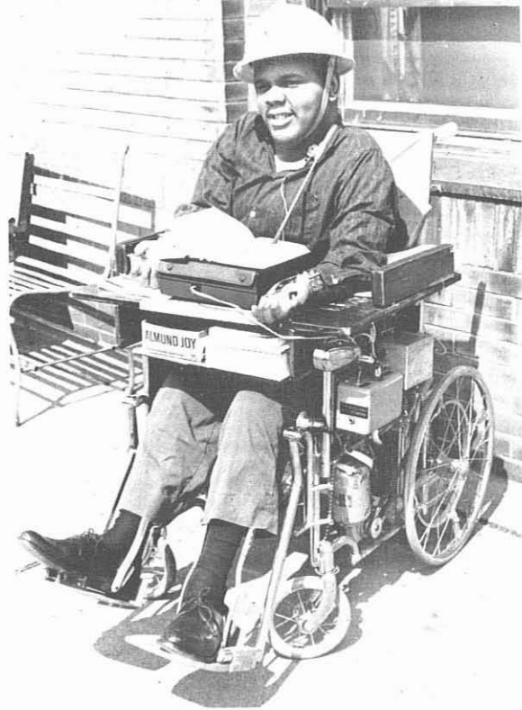
Bruce Lowe, polio quad, reviews his college textbooks at Goldwater Memorial Hospital residence. The control system in his hat is his electronic "genie" with which he drives the wheelchair, honks the horn, flashes his signal light and operates the tape recorder (under the book). Note the microphone in his lapel and the old fashioned non-electronic mouthstick for page-turning.
