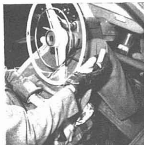
The driving position with the gloved right hand operating the accelerator.
