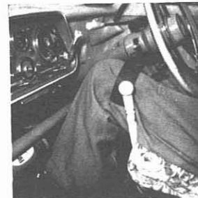
The foot brake is connected up to the white rod at the side of the driver. This is pushed forward to apply the brakes. The band over the knee prevents the leg from falling sideways and fouling the brake lever.
