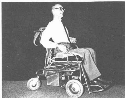
The switchbox (under Don's right hand) on the newer models now moves back and forth with the seat and the chair arms. This facilitates operation of switches by individuals with limited reach.
