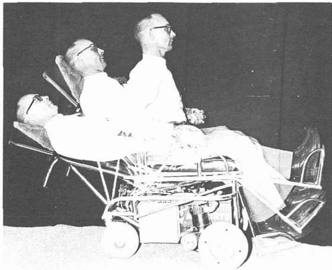
Multiple-exposure demonstrates the self-reclining ability and purpose of the Rugg Chair. (Note: the headrest adjusts automatically, dropping back when in the erect position.)
