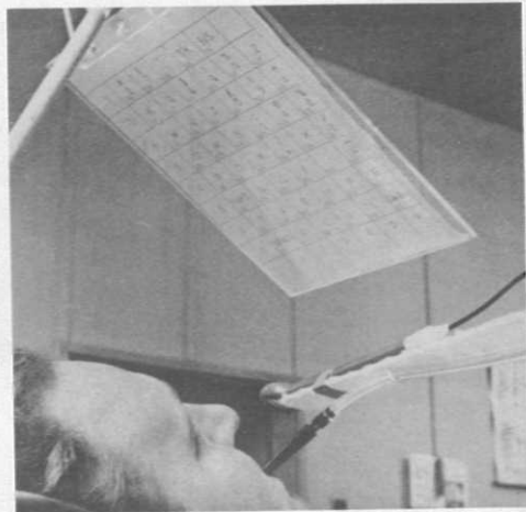
C. Close up of the chart which is the key to operating the electric typewriter by suck and blow.
