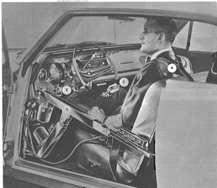
Ernest Trujillo demonstrates his automobile equipped with all automotive aids necessary for safe and independent driving by quad drivers. 1. Automolift: Wheelchair-to-Car Quadriplegic Lift. 2. Universal Hand Control. 3. Quadriplegic Steering Spinner. 4. Safety Harness.
